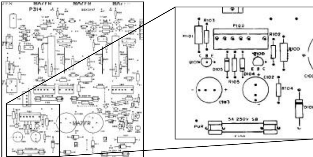
Remove the low voltage components from the highlighted area of the deflection board.
