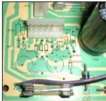
Remove the entire lead of each component from the holes, i.e., don't just "clip" them out. If there is any metal or residual solder on the top side of the deflection board, it could short out the LV2000 board when it's installed.
