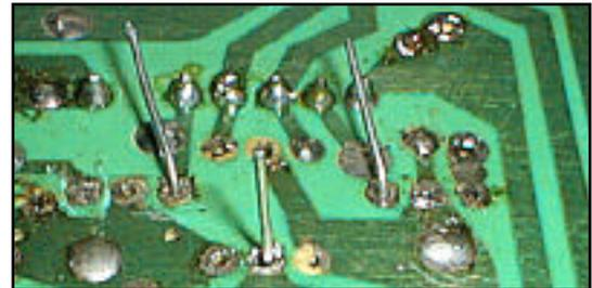
Solder the black wire into the top hole where resistors R101 came out of (the left hole marked with a square in the deflection board drawing above), and solder the red wire into the top hole where resistor R100 came out of (the right hole marked with a square in the deflection board drawing above).
