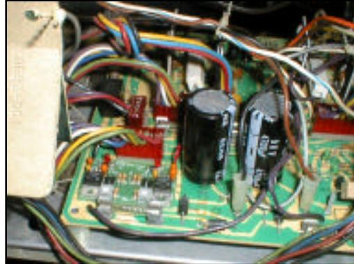
Once your game is on and the picture is displaying correctly, you may have to adjust the X and Y size, center, linearity, etc. to get the picture to be the same size as it was before the LV2000 was installed. This will happen since the voltage produced by the LV2000 will be slightly different than the voltage that was produced by the old low voltage components.
